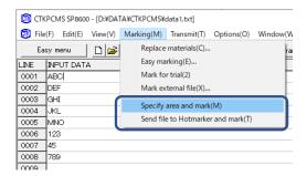
(9) After the conversion is completed, select "Marking" from the menu bar and choose "Specify area and mark" or "Send file to Hotmarker and mark" when start marking.
